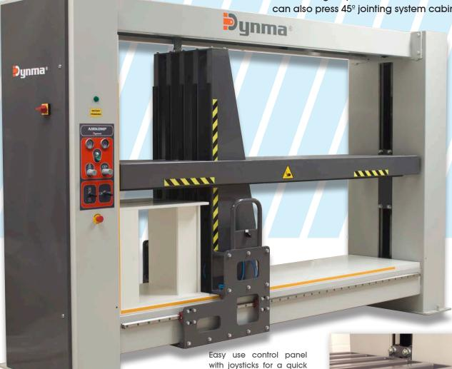
Platform and column are constructed with intercrossed steel pipes and covered with anti-friction strips for best sliding in pressing operation.
